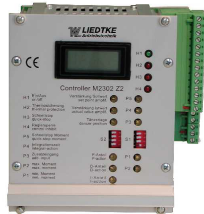
Picture: Controller M2302 with optional LC-Display and PID-regulator Z2
