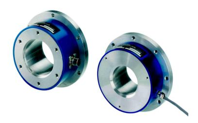
The torque sensor works independently from the speed and is used for static torque measurement. The installation position is arbitrarily and the measurement is made wear-free. The device is structured as reaction-torque sensor and is fixed on one side. According to the load direction of the torque, the sensor supplies via the measuring amplifier a signal of 0-10 VDC and 0-20 mA and that over the whole range of measuring.
