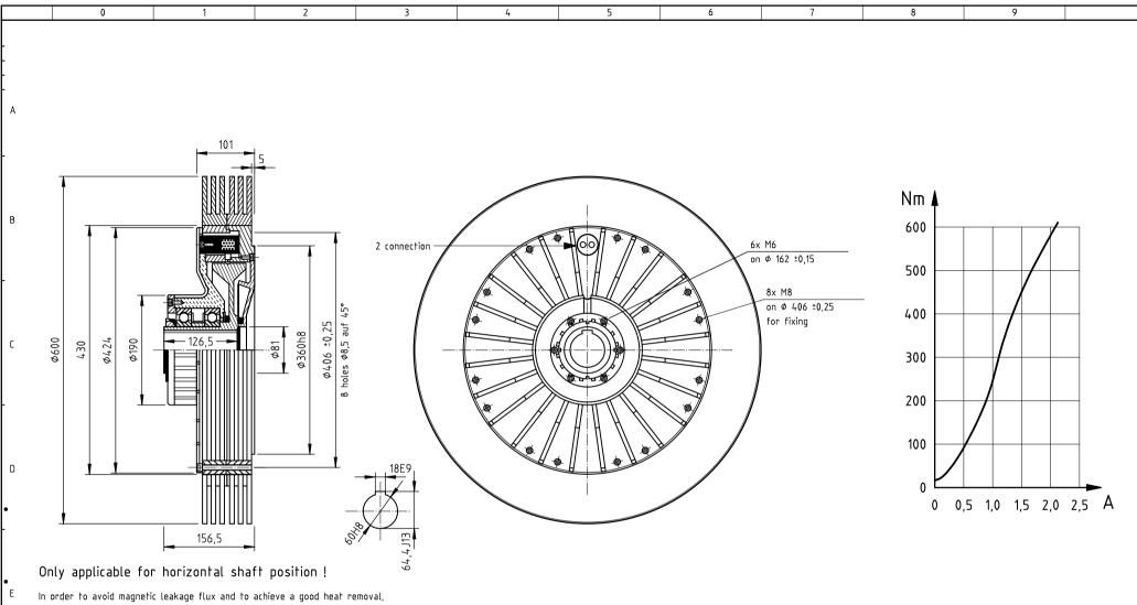
In order to avoid magnetic leakage flux and to achieve a good heat removal non-ferrous metals should be used for installation or attachment of auxiliary components (not for drive shaft).
