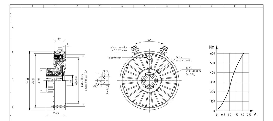
In order to avoid magnetic leakage flux and to achieve a good heat removal, non-ferrous metals should be used for installation or attachment of auxiliary components (not for drive shaft).
