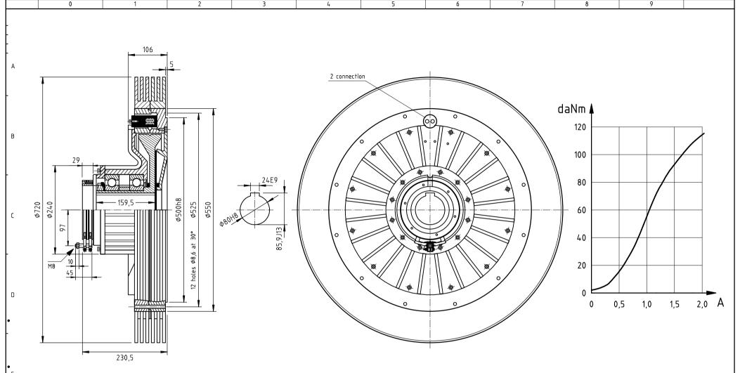
In order to avoid magnetic leakage flux and to achieve a good heat removal, non-ferrous metals should be used for installation or attachment of auxiliary components (not for drive shaft).
