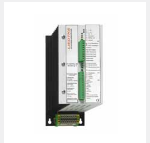
AC voltage regulator W3412.1S Motor voltage: 0 V–3 x 400 V AC Motor current: 0–12 A Available with options of DC braking and/or tension regulator
