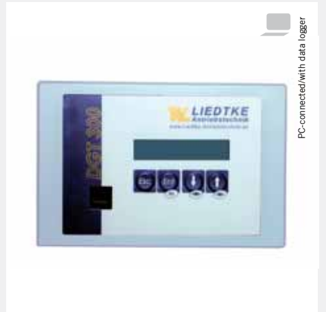
DGT 300 digital web tension controller for magnetic powder clutches and brakes, PID controller with direct or indirect tension control, taper control and inertia compensation control.
