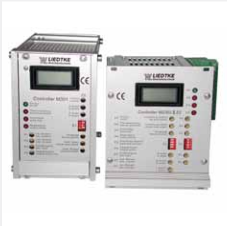
Constant current controllers M301(1A), 24 V AC or DC, M2302 II (2/3A), 230 V AC und M242 (2A) 24 V DC (no Fig.) available as an option with PID controller, display. Frontpanel for 19" rack.
