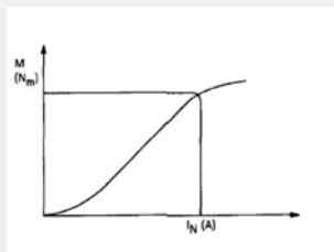
Diagram 1: The torque to be transmitted and the energising current behave are virtually in proportion to one another.
